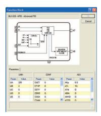
Online help shows detail diagrams of the internal function of the block when setting parameters. Help also includes information about valid ranges and options for each parameter.
